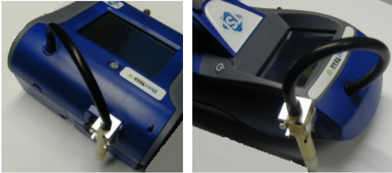
Figure 2-5: Installing Door-Oliver Cyclone
